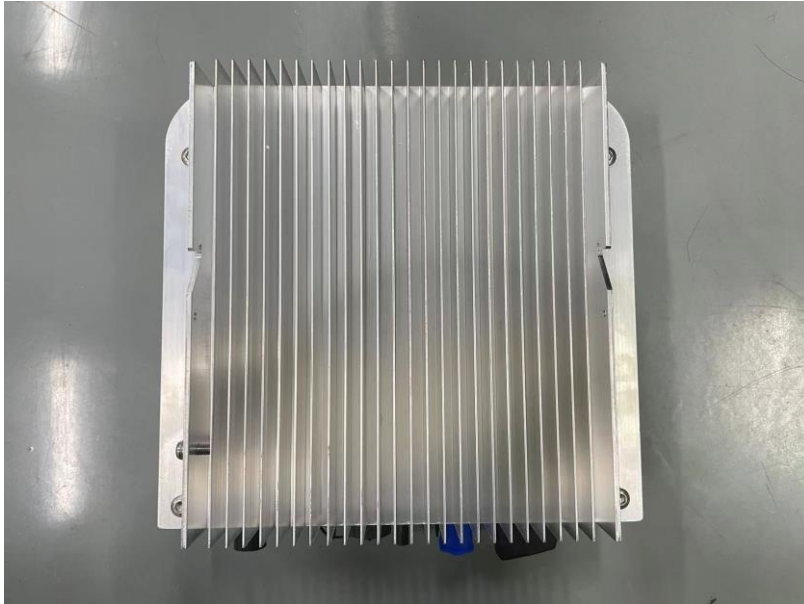
Back view of PV inverter
