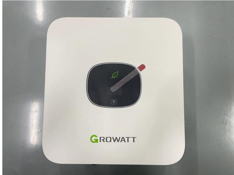
Front view of PV inverter
