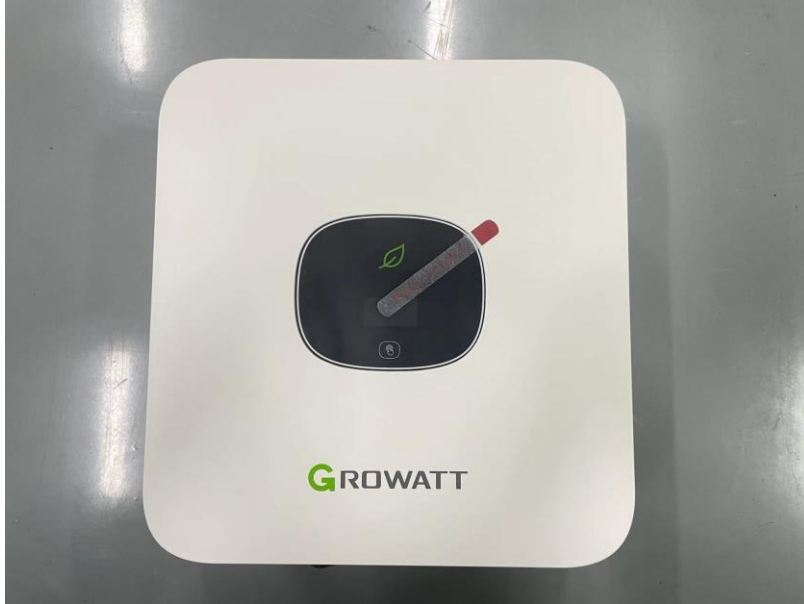
Front view of PV inverter
